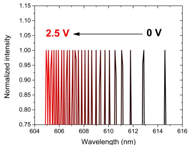
**Fig 2. Tuning the laser wavelength with a dc voltage**
