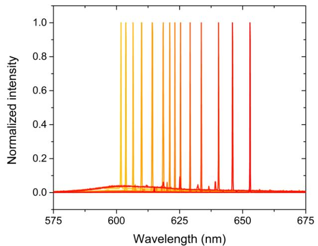
**Fig 1. Single mode tunable lasing over a wavelength range of 150 nm (Rhodamine 640 dye). The dye is pumped at  $\lambda = 532 \text{ nm}$  with  $\sim 300 \text{ pJ}$  pulses.**
