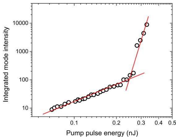
**Fig 3. Output intensity of the laser as a function of excitation pulse energy, showing a lasing threshold of 250 pJ.**
